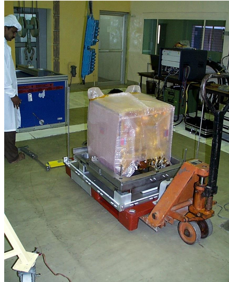
Micro satellite BIRD (with cover) fixed at mounting plate of the transport container [Foto: ISRO]
