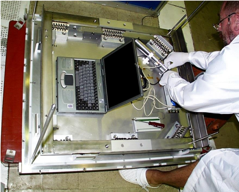
Integration of the shock recorder in the transport container of the BIRD satellite [photo: DLR ]
